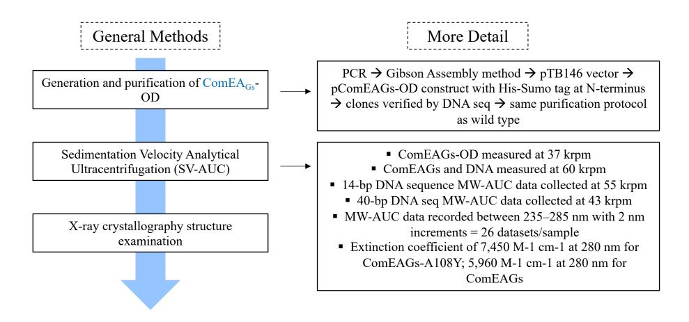
$\left(\frac{\partial C}{\partial t}\right)_r = \frac{-1}{r} \frac{\partial}{\partial r} \left[s\omega^2 r^2 C\right]$  $\partial C$ (Lamm Equation)
